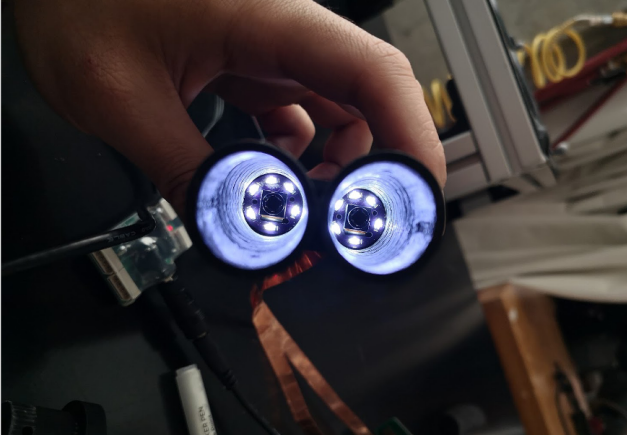
Figure 6. View inside the HSA, where our custom-made LED board, mounted at the tip, provides internal lighting for the cameras.
