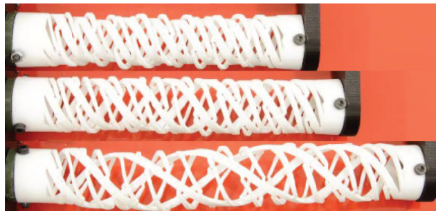
Figure 1. HSAs are polymer tubes with a unique pattern that makes them extend when twisted at the end [6].
